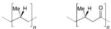
Fig. 3. Representation of the monomeric units of polypropylene (left) vs. propylene-CO copolymers (right)
